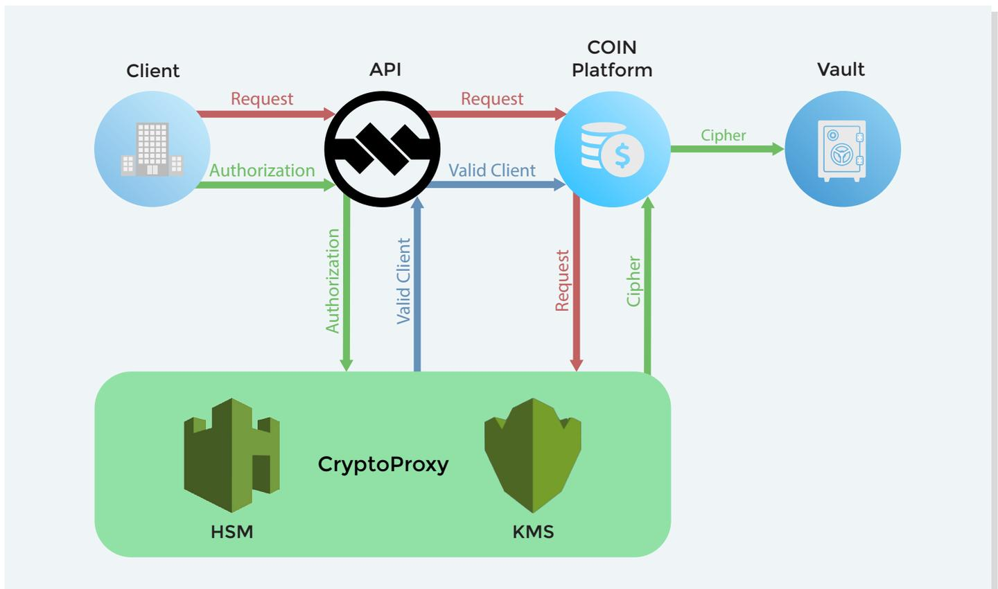
When a client application makes a request to Modo, CryptoProxy routes the request to the appropriate key-store for validation. Once validated, the request is released to the Modo platform and CryptoProxy provides the Modo platform with the keys needed to access Vault information to be used for processing.
